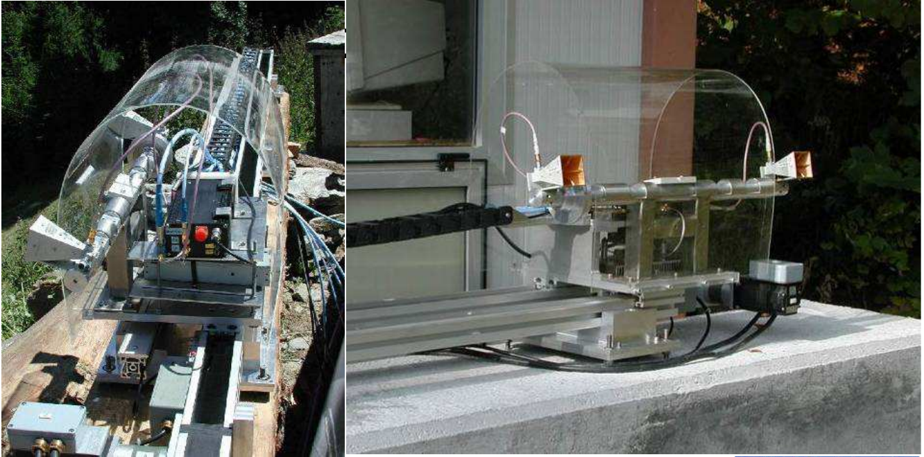
Portable SAR apparatus known as LISA ( Linear Synthetic Aperture Radar ), developed by the Joint Research Centre of the European Commission
